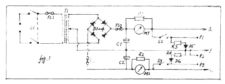
The circuit diagram shows no fancy tricks are used. An IEC mains connector on the back panel included a mains switch and fuse holder. If like me you use a toroidal transformer use a slow-blow fuse here as the inrush current, though short lived, can be considerable. My transformer was a 0-15, 0-15V 120VA from Electrovalue. The rectifier was assembled on its own PCB with two fuses.
